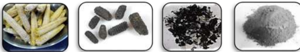
Figure 2: Corn Cob Ash Preparation Sequence. Source: Swami et al., (2022)
