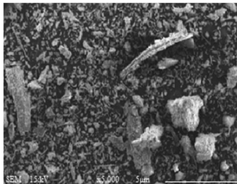
Figure 4: Microstructure of Corn Cob Ash, Source: Pharm et al., 2021.
